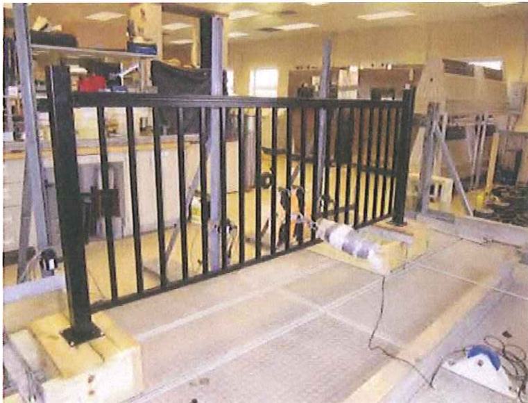
Photo No. 2 In-Fill Load Test at Bottom of Two Pickets
