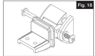
Adjust the top stair bracket to match the stair angle. Align the top beam with the brackets and mark both ends (Fig. 19). Cut at these marks and test for proper fit.
