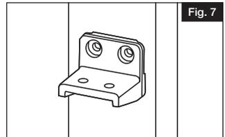
**NOTE:** Mounting hardware included in bracket kits is comprised of (8) 1½" screws and (4) 1⅝" screws. Be sure to use 1½" screws when installing brackets to the post and keep longer 1⅝" screws for installing top rail. 1⅝" are specifically designed to be longer and lock top rail in place at the end of installation.
