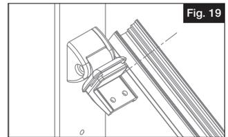
Measure the length of the top beam and cut the top rail (sold separately) to the same length. Insert the top channel into the top rail and ensure both ends are aligned. Disassemble both top brackets by removing the hinge bolt. Align the stair bracket with the rail end (Fig. 20). Using the pre-drilled holes as a guide, drill through the railing using a  $\frac{1}{8}$ " bit as shown, (Fig. 21) being careful not to drill through the top of the top rail (circled with dotted lines Fig. 21).
