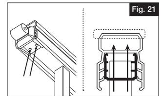
For each bracket, drive two #8 x  $1\frac{1}{2}$ " painted pan head screws through the pre-drilled holes locking the bracket, top channel and top rail together. After the top rail is secured on both ends, slide the brackets into the bases on the posts and lock the assembly using the base covers and hinge bolts provided.
