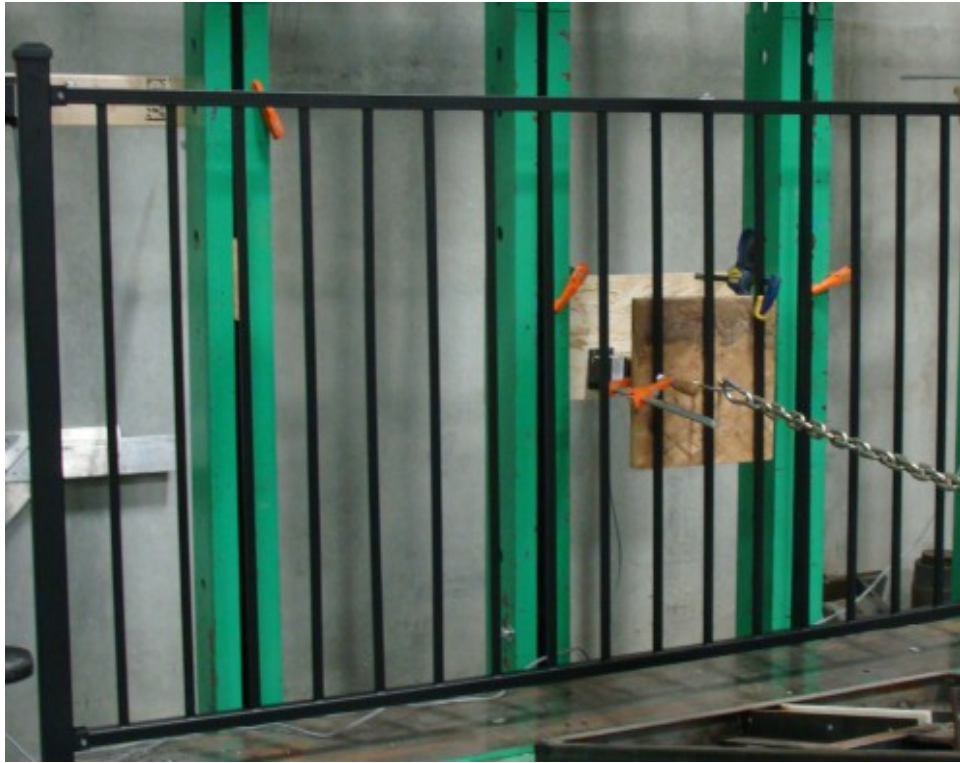
PHOTO 7: 50 lbf Load – Infill
