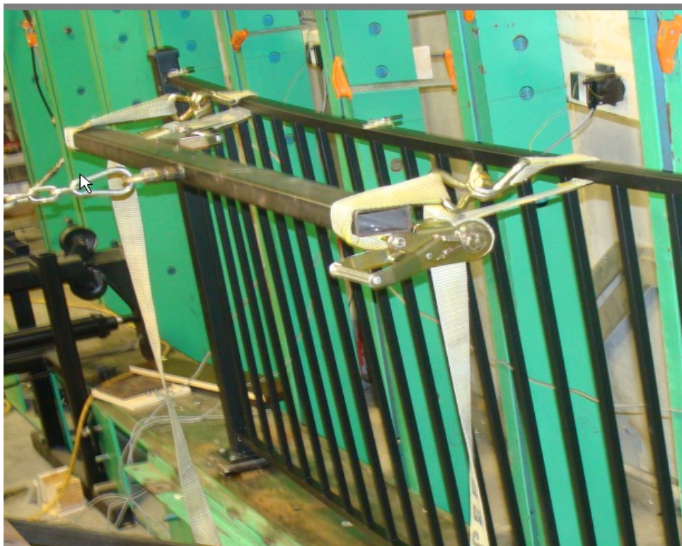
PHOTO 8: 400 lbf (50 plf Uniform) Load Applied – Horizontal
