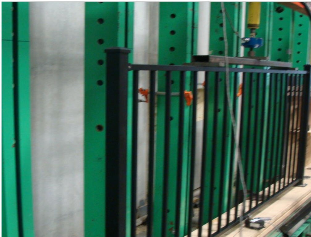
PHOTO 4: 400 lbf (50 plf Uniform) Load Applied – Vertical
