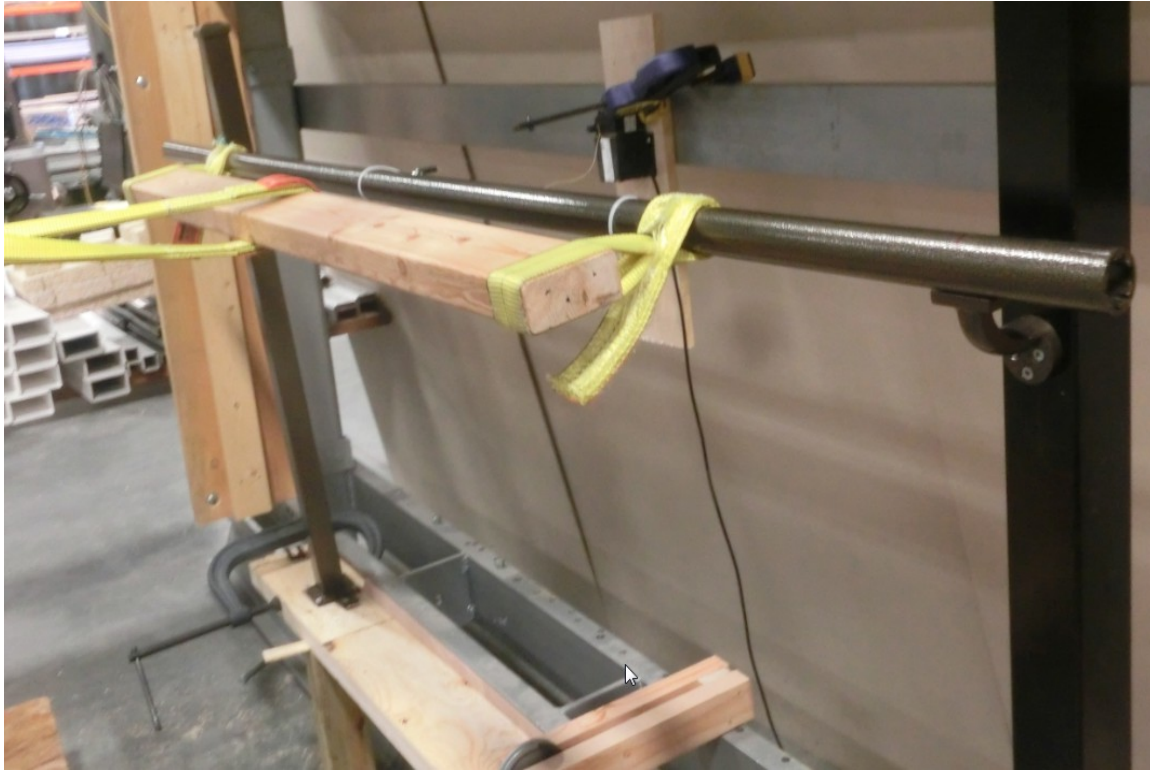
Photo 7: Typical Setup for Horizontal Uniform Load
