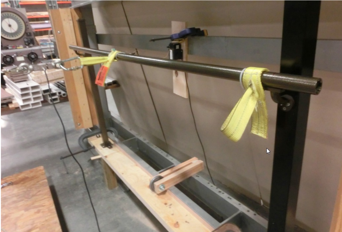
Photo 5: Typical Setup for Horizontal Concentrated Load at Midspan
