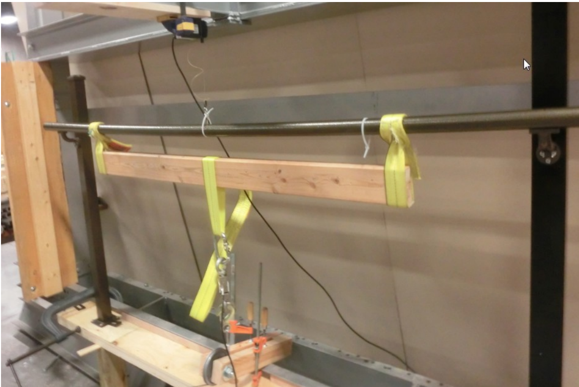
Photo 8: Typical Setup for Vertical Concentrated Load at Midspan
