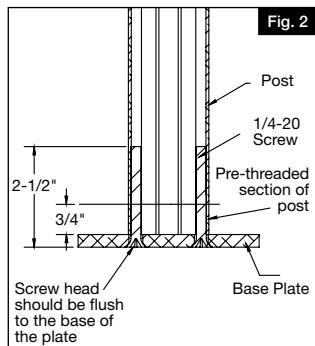
Attach post/base assembly to surface using appropriate  $\frac{1}{8}$ " fasteners.
