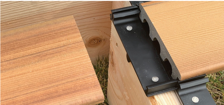
Additional framing may be needed for inline boards (Step-Clips cannot be shared by inline boards).
