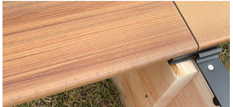
Sister or add framing where butt joints occur then trim a single Step-Clip strip section to accommodate each board and attach separately to the additional framing.
