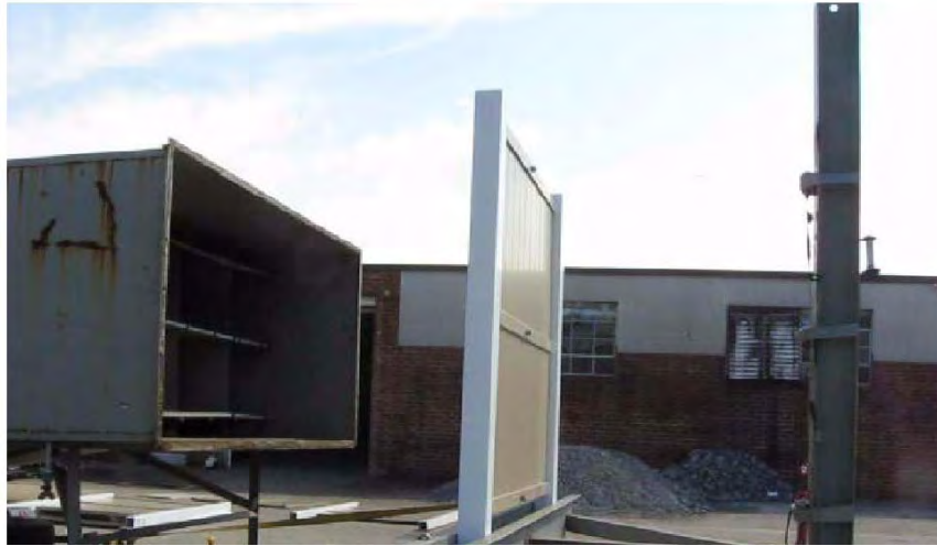
Photo No. 1 Dynamic Wind Test Setup - Cameron Fence Panel
