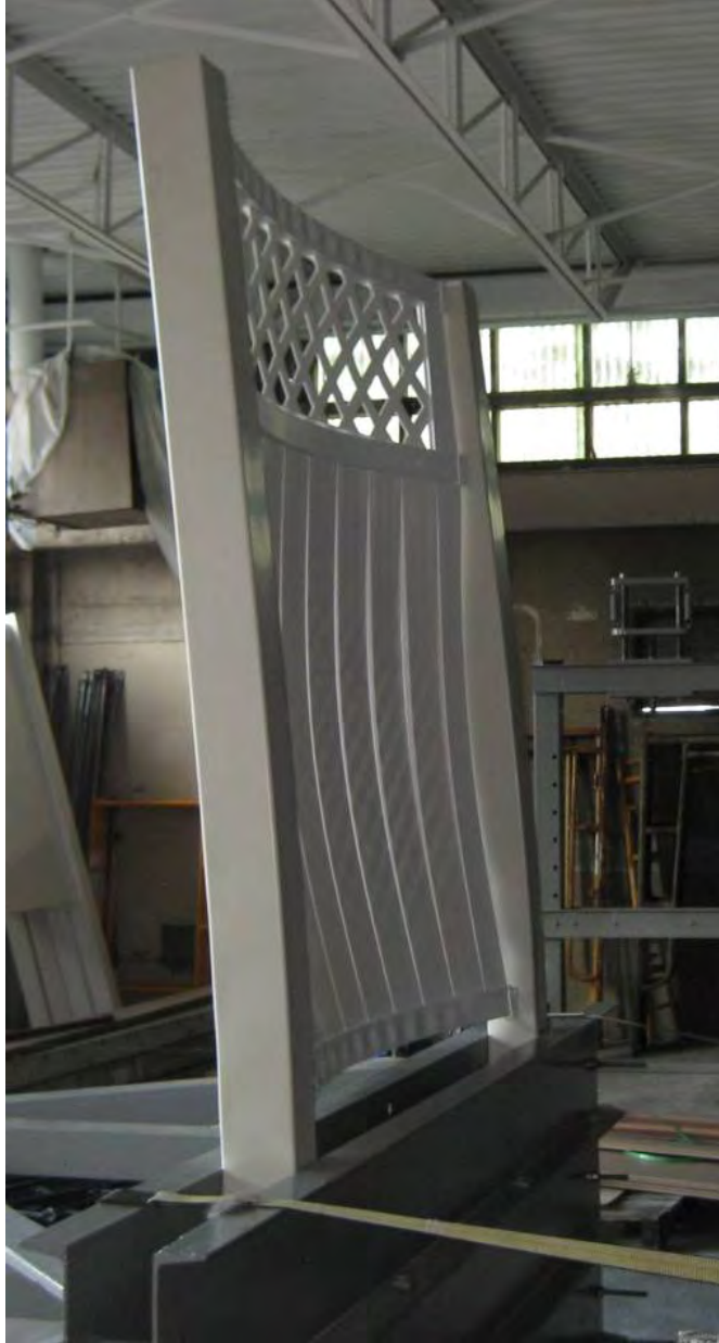
Photo No. 3 Halifax Fence Panel During Dynamic Wind Test
