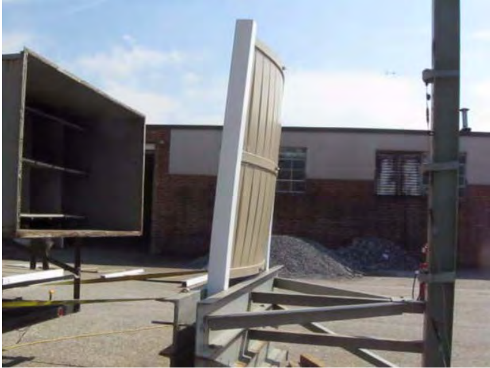
Photo No. 4 Cameron Fence Panel During Dynamic Wind Test
